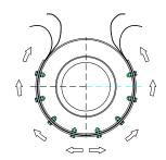
For open ended expansion joints with circular cross sections start from the opposite side of the splice and work in both directions towards the splice
