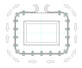
For open ended expansion joints with rectangularcross sections start from the corners. Spread out material equally between the fasteners
